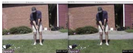
Figure 5. CompressHD (shown on the right) didn't insert keyframes at scene changes, which created problems with this scene change.
